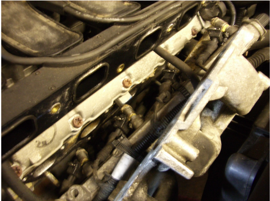
Figure 2 Removing the Lower Manifold exposing the detached fuel rail
