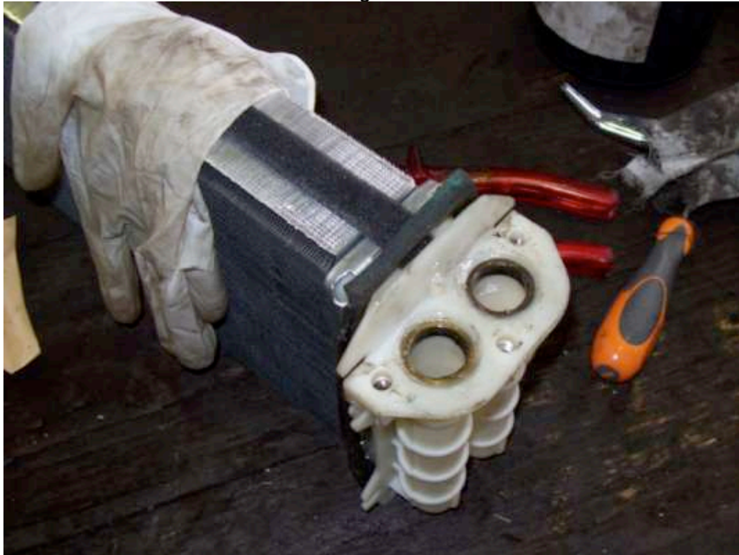
NEW HEATER MATRIX with O – rings
